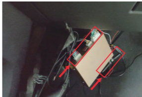
26. 将CarPlay的WiFi天线和蓝牙天线连接到盒子上；将LVDS线和主线的白色插头连接到盒子上 Connect CarPlay's Bluetooth antenna, WiFi antenna and usb cable to the box; Connect the CarPlay LVDS cable and the white plug of the main cable to the box
