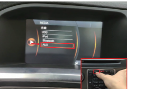
2. 通过原车MEDIA键进入媒体界面，选择AUX Enter the media interface of the original car system through the MEDIA button, select AUX
