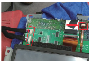
14. 将CarPlay的LVDS先连接到PCB板上，并将屏幕原来的排线重新接上 Connect the CarPlay LVDS cable to the PCB board; And reconnect the original flat cable of the screen
