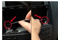
3. Pick up the clips on the screw hole area when take out the head unit.
