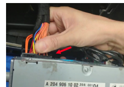
14. Insert the male side of the iSmart auto box 48PIN harness into head unit.
