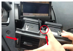
1. Remove the air conditional panel, note the connector behind it
