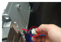
5. Note that there is a plug on the side of the head unit, which needs to be pulled out.
