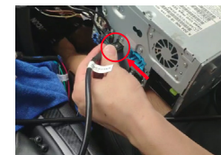
13. Insert another side of iSmart auto box LVDS IN cable into head unit.
