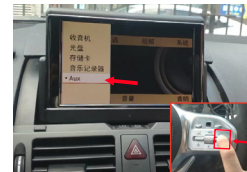
14. Enter the audio interface - choose AUX, Long press phone-ending button to switch to carplay interface.
