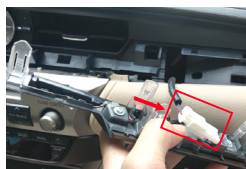
6. Take out the air conditioner trim panel, pay attention to the plug behind the trim panel
