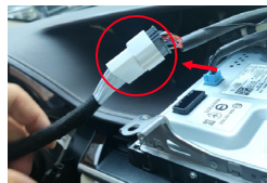
4. Take out the CarPlay screen adapter cable and connect it to the plug of the original car's screen
