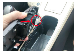
11. Remove the knob panel and pull out the plug behind the knob panel.
