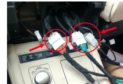
15. Take out CarPlay's power adapter cable, CAN adapter cable and audio adapter cable to connect with the original car
