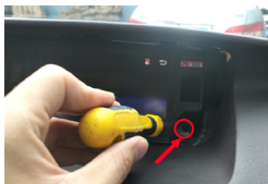
1. Take out the trim of the screen and remove the screws on the screen
