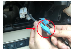
14. Connect the Limcet CarPlay video cable with the video cable of the original car
