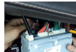
17. Reconnect the CarPlay plug and the original car's plug to the original car head unit
