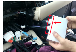
16. Connect the white plugs of the CarPlay main cable and video cable to the box, and connect the WiFi antenna to the box
