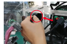
5. Take out the CarPlay audio cable and connect the CarPlay audio cable to the original car head
