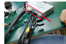
10. Connect the plugs of the CarPlay main cable, video cable and USB cable to the box, and connect the CarPlay antenna to the box
