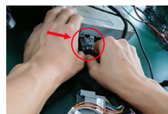
5. Connect the main power cord of iSmart CarPlay to the original car head unit
