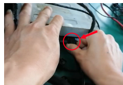
2. Connect the LVDS cable of iSmart CarPlay to the head unit
