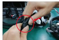
2. Take out the LVDS cable of iSmart CarPlay and connect it with the video cable of the original car
