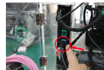
1. Unplug the video cable behind the head unit
