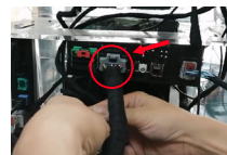
8. Connect the main power cord of iSmart CarPlay to the original car head
