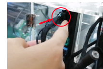
4. Unplug the audio cable behind the head unit of the original car
