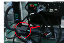
6. Connect the audio cable of CarPlay with the audio cable of the original car
