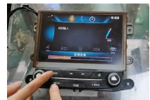
11. Enter the media interface in the original car system and select AUX
