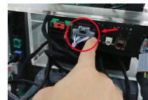
7. Unplug the power cord behind the head unit
