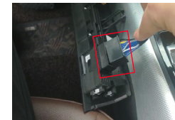
13. Insert the iSmart box air conditional cable into original car air conditional panel
