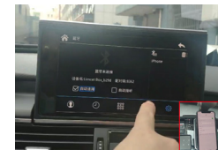
19. At the Carplay system Bluetooth interface, you can find the iSmart box Bluetooth name and pairing code.
