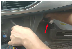
7. Take iSmart box 48pin harness cable, and get it through ACC area to glove box area
