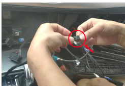
9. Connect the 4PIN cable on LVDS cable with original car LVDS cable.
