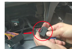
12. Connect the iSmart box air conditional cable with original car air conditional panel connector
