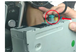
14. Insert the iSmart box LVDS cable into multimedia box
