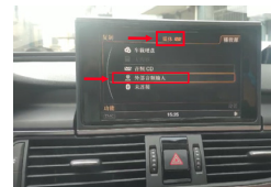
17. Click MEDIA to enter original car media interface, choose external audio input.
