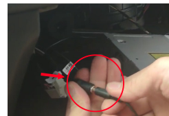
11. Connect the iSmart box microphone cable
