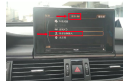
1. Click MEDIA to enter original car media interface, choose external audio input.
