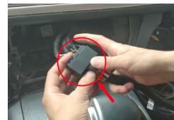
10. Connect the iSmart 48pin cable with original car 48pin connector
