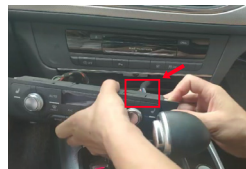
3. Remove off the air conditional panel with plastic mover tool, be note on the connectors behind it. Disconnect the connectors
